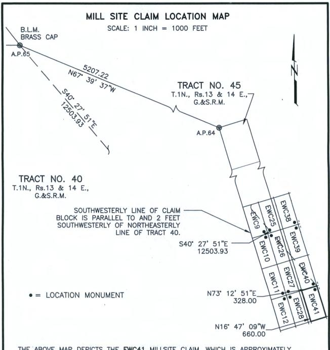
THE ABOVE MAP DEPICTS THE **EWC41** MILLSITE CLAIM, WHICH IS APPROXIMATELY LOCATED IN THE NE QUARTER OF PROTRACTED SECTION 18, AND IN THE NW QUARTER OF PROTRACTED SECTION 17, IN UNSURVEYED TOWNSHIP 1 NORTH, RANGE 14 EAST OF THE GILA AND SALT RIVER MERIDIAN, GILA COUNTY, ARIZONA. THE TOTAL AREA IS 4.970 ACRES, MORE OR LESS.
