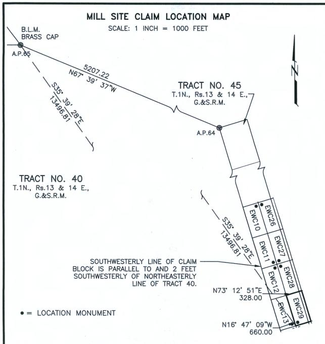
THE ABOVE MAP DEPICTS THE **EWC29** MILLSITE CLAIM, WHICH IS APPROXIMATELY LOCATED IN THE NE QUARTER OF PROTRACTED SECTION 18, AND IN THE NW QUARTER OF PROTRACTED SECTION 17, IN UNSURVEYED TOWNSHIP 1 NORTH, RANGE 14 EAST OF THE GILA AND SALT RIVER MERIDIAN, GILA COUNTY, ARIZONA. THE TOTAL AREA IS 4.970 ACRES, MORE OR LESS.
