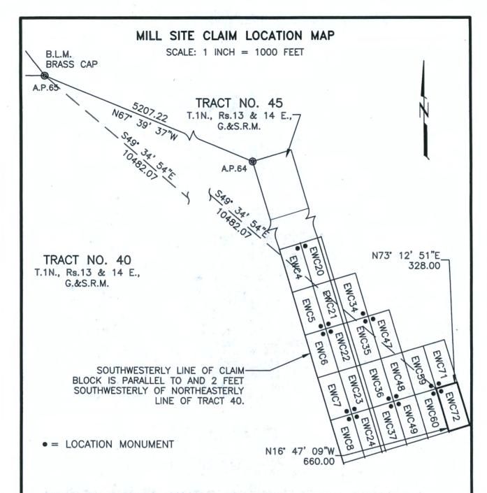
THE ABOVE MAP DEPICTS THE **EWC72** MILLSITE CLAIM, WHICH IS APPROXIMATELY LOCATED IN THE SE & NE QUARTERS OF PROTRACTED SECTION 7, AND IN THE SW & NW QUARTERS OF PROTRACTED SECTION 8, IN UNSURVEYED TOWNSHIP 1 NORTH, RANGE 14 EAST OF THE GILA AND SALT RIVER MERIDIAN, GILA COUNTY, ARIZONA. THE TOTAL AREA IS 4.970 ACRES, MORE OR LESS.
