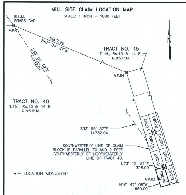
THE ABOVE MAP DEPICTS THE **EWC16** MILLSITE CLAIM, WHICH IS APPROXIMATELY LOCATED IN THE SE QUARTER OF PROTRACTED SECTION 18, AND IN THE SW QUARTER OF PROTRACTED SECTION 17, IN UNSURVEYED TOWNSHIP 1 NORTH, RANGE 14 EAST OF THE GILA AND SALT RIVER MERIDIAN, GILA COUNTY, ARIZONA. THE TOTAL AREA IS 4.970 ACRES, MORE OR LESS.
