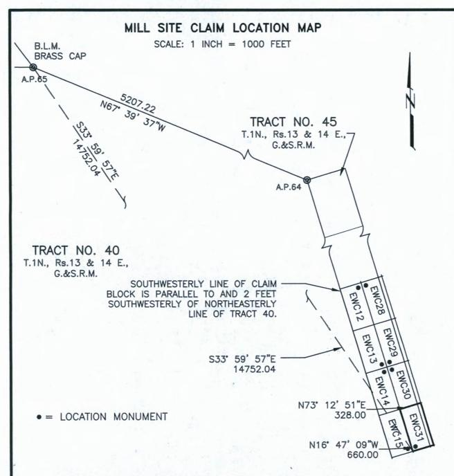
THE ABOVE MAP DEPICTS THE **EWC31** MILLSITE CLAIM, WHICH IS APPROXIMATELY LOCATED IN THE NE QUARTER OF PROTRACTED SECTION 18, AND IN THE NW & SE QUARTERS OF PROTRACTED SECTION 17, IN UNSURVEYED TOWNSHIP 1 NORTH, RANGE 14 EAST OF THE GILA AND SALT RIVER MERIDIAN, GILA COUNTY, ARIZONA. THE TOTAL AREA IS 4.970 ACRES, MORE OR LESS.
