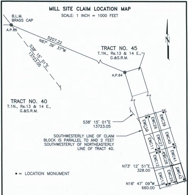
THE ABOVE MAP DEPICTS THE **EWC42** MILLSITE CLAIM, WHICH IS APPROXIMATELY LOCATED IN THE NE QUARTER OF PROTRACTED SECTION 18, AND IN THE NW QUARTER OF PROTRACTED SECTION 17, IN UNSURVEYED TOWNSHIP 1 NORTH, RANGE 14 EAST OF THE GILA AND SALT RIVER MERIDIAN, GILA COUNTY, ARIZONA. THE TOTAL AREA IS 4.970 ACRES, MORE OR LESS.
