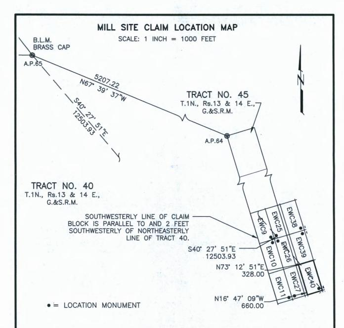
THE ABOVE MAP DEPICTS THE **EWC40** MILLSITE CLAIM, WHICH IS APPROXIMATELY LOCATED IN THE SE QUARTER OF PROTRACTED SECTION 7, AND IN THE NE QUARTER OF PROTRACTED SECTION 18, IN UNSURVEYED TOWNSHIP 1 NORTH, RANGE 14 EAST OF THE GILA AND SALT RIVER MERIDIAN, GILA COUNTY, ARIZONA. THE TOTAL AREA IS 4.970 ACRES, MORE OR LESS.
