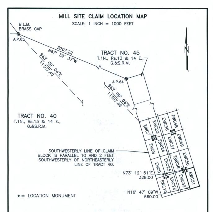
THE ABOVE MAP DEPICTS THE **EWC51** MILLSITE CLAIM, WHICH IS APPROXIMATELY LOCATED IN THE SE QUARTER OF PROTRACTED SECTION 7, AND IN THE SW QUARTER OF PROTRACTED SECTION 8, IN UNSURVEYED TOWNSHIP 1 NORTH, RANGE 14 EAST OF THE GILA AND SALT RIVER MERIDIAN, GILA COUNTY, ARIZONA. THE TOTAL AREA IS 4.970 ACRES, MORE OR LESS.
