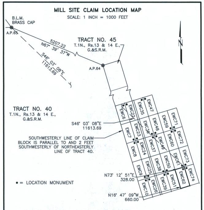
THE ABOVE MAP DEPICTS THE **EWC62** MILLSITE CLAIM, WHICH IS APPROXIMATELY LOCATED IN THE SE QUARTER OF PROTRACTED SECTION 7, AND IN THE SW QUARTER OF PROTRACTED SECTION 8, IN UNSURVEYED TOWNSHIP 1 NORTH, RANGE 14 EAST OF THE GILA AND SALT RIVER MERIDIAN, GILA COUNTY, ARIZONA. THE TOTAL AREA IS 4.970 ACRES, MORE OR LESS.
