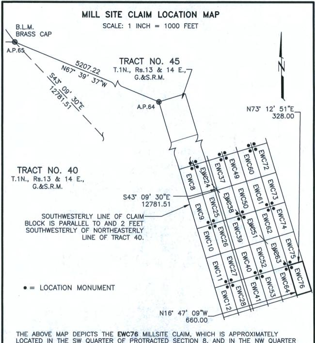
THE ABOVE MAP DEPICTS THE **EWC76** MILLSITE CLAIM, WHICH IS APPROXIMATELY LOCATED IN THE SW QUARTER OF PROTRACTED SECTION 8, AND IN THE NW QUARTER OF PROTRACTED SECTION 17, IN UNSURVEYED TOWNSHIP 1 NORTH, RANGE 14 EAST OF THE GILA AND SALT RIVER MERIDIAN, GILA COUNTY, ARIZONA. THE TOTAL AREA IS 4.970 ACRES, MORE OR LESS.
