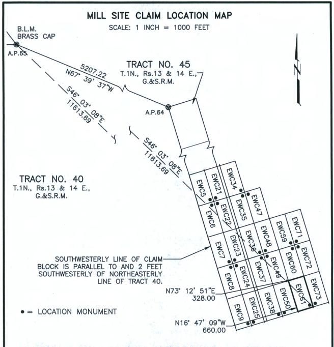
THE ABOVE MAP DEPICTS THE **EWC61** MILLSITE CLAIM, WHICH IS APPROXIMATELY LOCATED IN THE SE QUARTER OF PROTRACTED SECTION 7, AND IN THE SW QUARTER OF PROTRACTED SECTION 8, IN UNSURVEYED TOWNSHIP 1 NORTH, RANGE 14 EAST OF THE GILA AND SALT RIVER MERIDIAN, GILA COUNTY, ARIZONA. THE TOTAL AREA IS 4.970 ACRES, MORE OR LESS.
