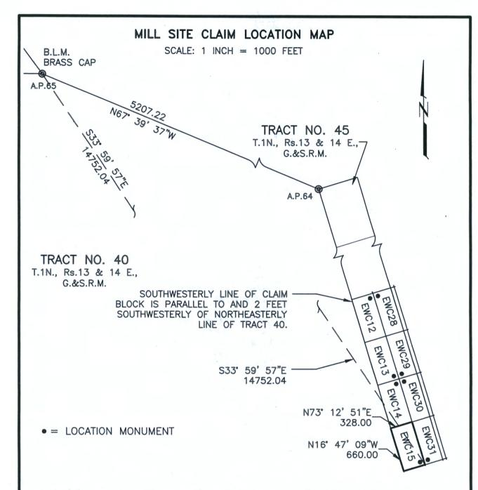
THE ABOVE MAP DEPICTS THE **EWC15** MILLSITE CLAIM, WHICH IS APPROXIMATELY LOCATED IN THE NE & SE QUARTERS OF PROTRACTED SECTION 18, AND IN THE NW & SW QUARTERS OF PROTRACTED SECTION 17, IN UNSURVEYED TOWNSHIP 1 NORTH, RANGE 14 EAST OF THE GILA AND SALT RIVER MERIDIAN, GILA COUNTY, ARIZONA. THE TOTAL AREA IS 4.970 ACRES, MORE OR LESS.
